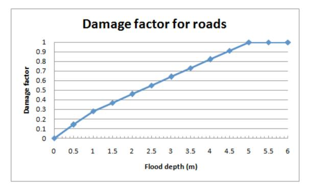
*Figure 27.* Damage factor for roads (with no storm and water flow rate of 0 m/s) (Meidinger, 2010).
