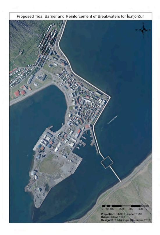
Figure 41. Proposed tidal barrier for Ísafjörður.
