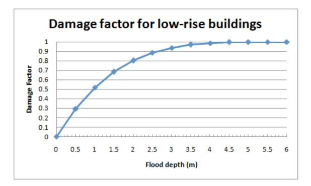
*Figure 26.* Damage factor for low-rise housing (with no storm and water flow rate of 0 m/s) (Meidinger, 2010).
